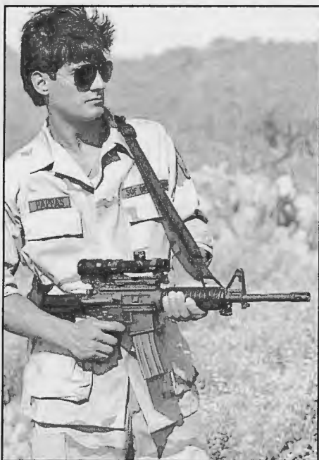
JFS Inc. patrol sling installed on M16A3 M4 Carbine permits waist-level carry and instant target acquisition with aimed fire from the shoulder.
